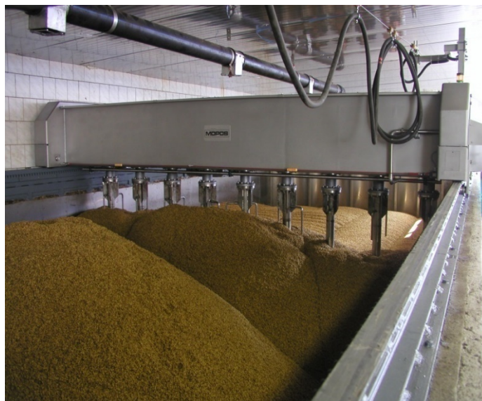
Figure 7 | Photo of Pneumatic Germination Box.
